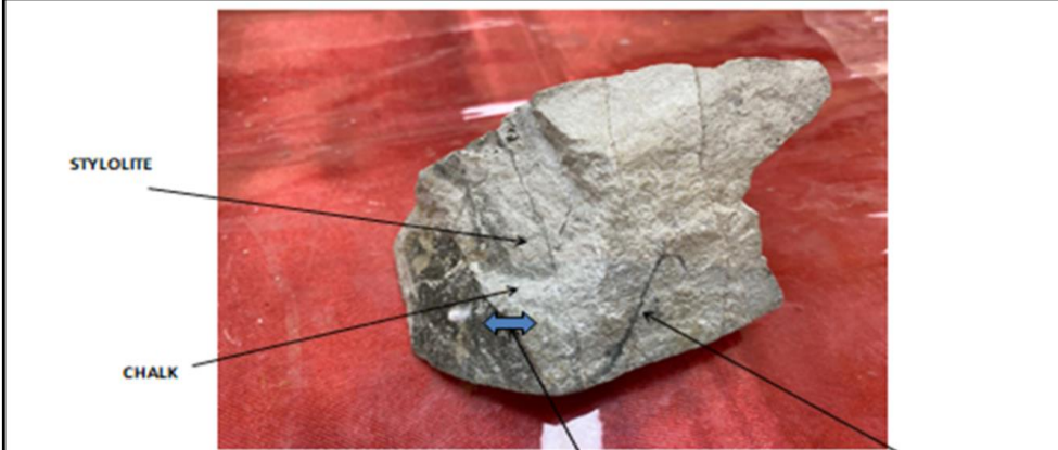
MASSIVE & LAMINATED DOLOSTONE LIGHT TO MEDIUM GREY, DARK GREY CRYSTALLINE FILLED FRACTURED PYRITIZED
